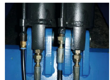
Figure19fixing position of end switch
